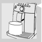
5 Place a large container (1.5 l) under both the steam/hot water wand and the dispensing spout.
