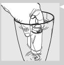
2 Remove the "INTENZA+" water filter from its packaging, immerse it vertically (with the opening positioned upwards) in cold water and gently press the sides so as to let the air bubbles out.
