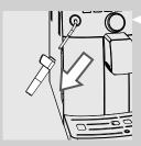
2 Remove the Classic Milk Frother and the "Intenza+" water filter (if installed).
