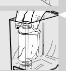
4 Insert the filter into the empty water tank. Press it down until it cannot move any further.
