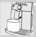
7 The steam/hot water wand ( button steady on) and the dispensing spout ( button steady on) start dispensing the descaling solution.
